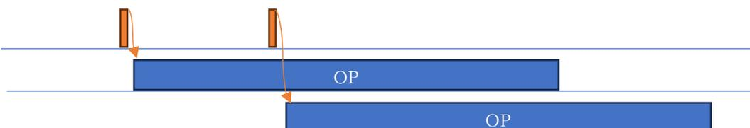
P3 : Relay will turn ON for time OP after getting a trigger signal and then turn relay OFF. Module will reset and stop timing if it gets a trigger signal again during delay time OP.
