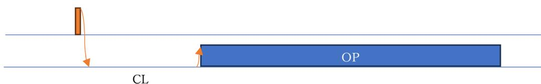
P5 : Relay will turn ON for time OP after getting a trigger signal and then relay will turn OFF for time CL and then loops the above action. Relay will turn OFF and stop timing if it gets a trigger signal again during the loop.
