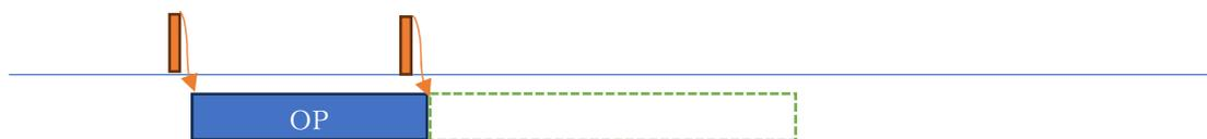
P4 : Relay will turn OFF for time CL after getting a trigger signal and then relay will turn ON for time OP. Relay will turn OFF after finish timing.
